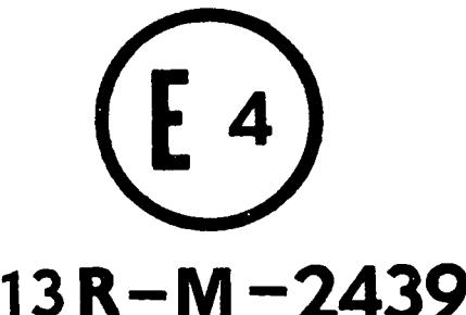
The above approval mark affixed to a vehicle of categories M<sub>2</sub> and M<sub>3</sub> shows that, pursuant to Regulation No. 13, the vehicle type concerned has with regard to braking, been approved in the Netherlands (E4) under approval number 2439 and that it has undergone the type-II *bis* test.
