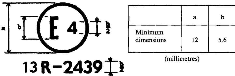
The above approval mark affixed to a vehicle shows that, pursuant to Regulation No. 13, the vehicle type concerned has, with regard to braking, been approved in the Netherlands (E4) under approval number 2439. For vehicles of categories M<sub>2</sub> and M<sub>3</sub>, this mark means that that type of vehicle has undergone type-II test.
